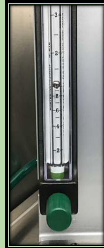
Flowmeter Set to 1 L/min
