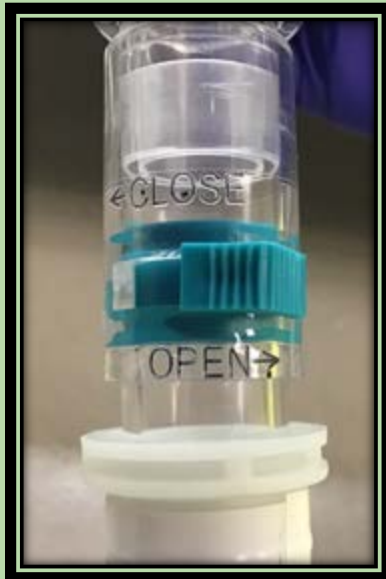
Pop-off valve open and internal view
