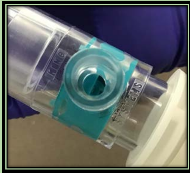
Pop-off valve open and internal view
