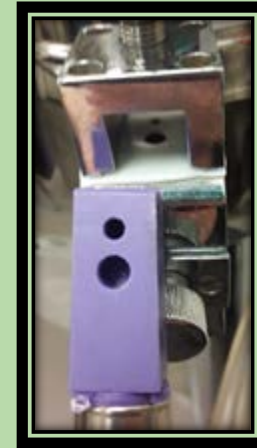
Holes in filling key will line up with holes in vaporizer port during proper placement
