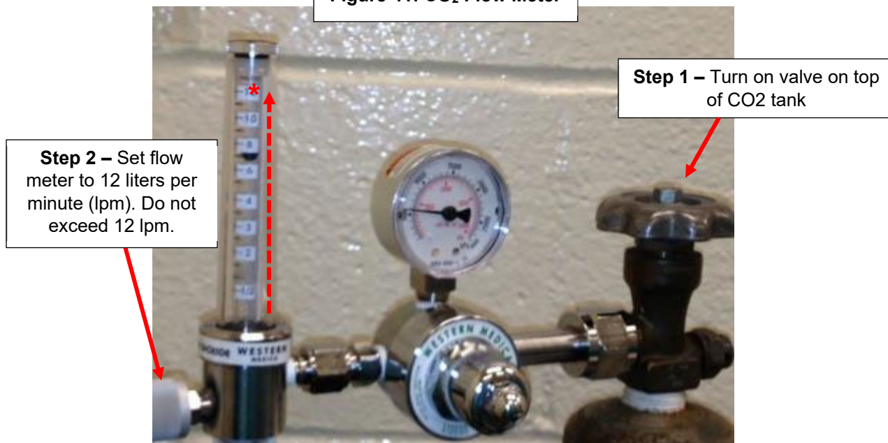
Figure 41: CO 2 Flow Meter
